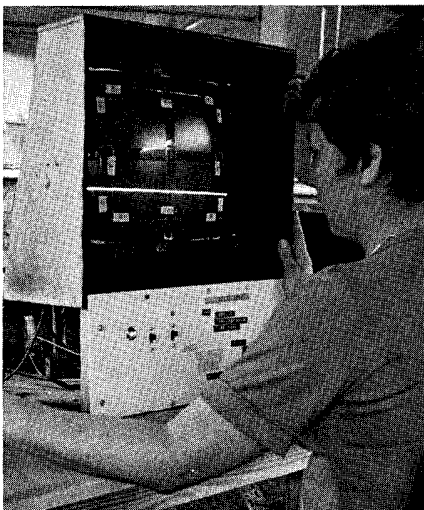
Four-Line Scanner used in testing yokes.
