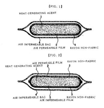
Tsuji's Figures 1 and 2 above depict sectional views of the disclosed warming apparatus including heat generating agent 1, air permeable film 2, rayon non-woven fabric 3, air impermeable bag 4, and air impermeable film 5 (pp. 6-7).
