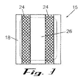
Figure 3 above depicts a plan view of a bag layer 15 of the claimed warming apparatus, in which the bag layer comprises an air permeable surface area 24 and an air impermeable surface area 26 (col. 2, ll. 47-48; col. 4, ll. 33-36).
