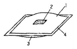
Koiso's Figure 1 above depicts an exothermic body, wherein the body includes air impermeable films 1 and 3, which are bonded together at their peripheral edges 4, and microscopic pore film 2 that forms an air permeable portion (pp. 5-6).
