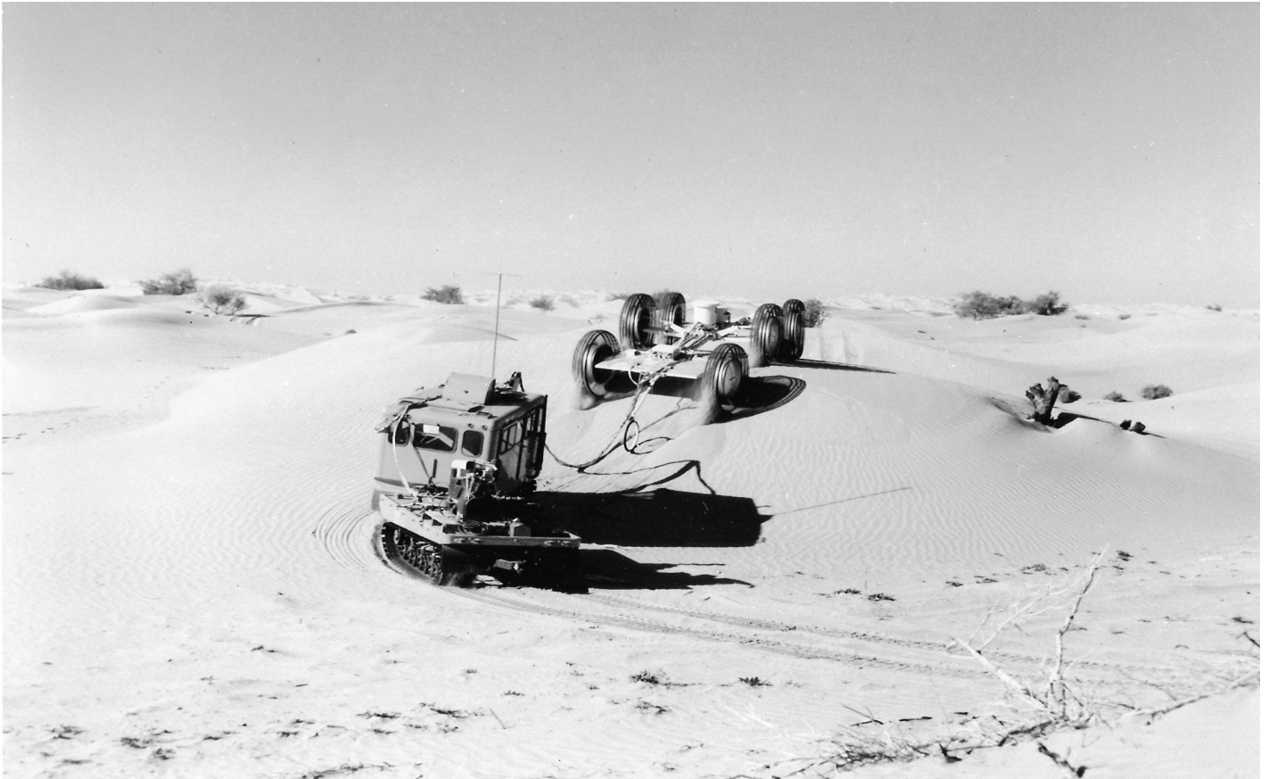
This photo shows some of the Yuma Test Areas that we considered to be representative of the the typical Maria area. with no debris from a nearby small craters. This shows the General Motors vehicle in a mobility test.
