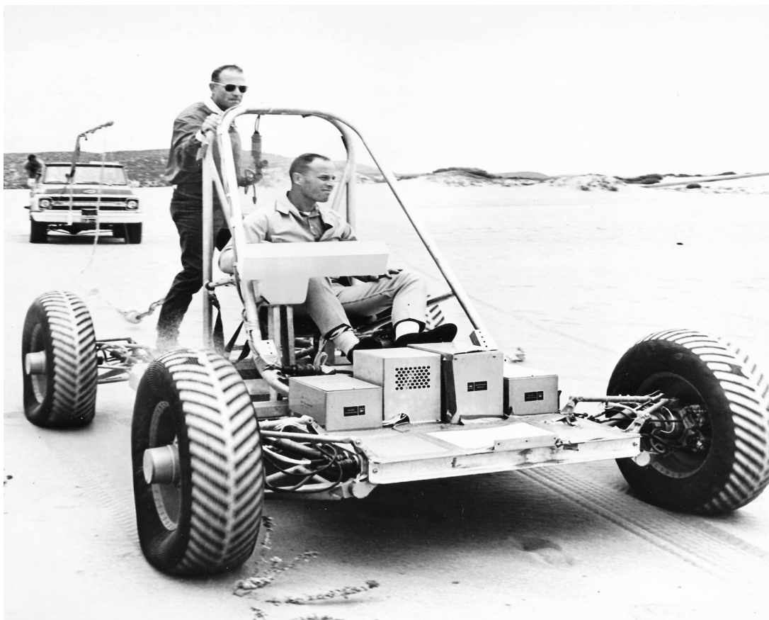
This is a photo of the Bendix Mobility Test Article that were developed for lunar mobility studies of large Lunar Rovers. It was also used for human factors and mobility evaluations here at MSFC.
