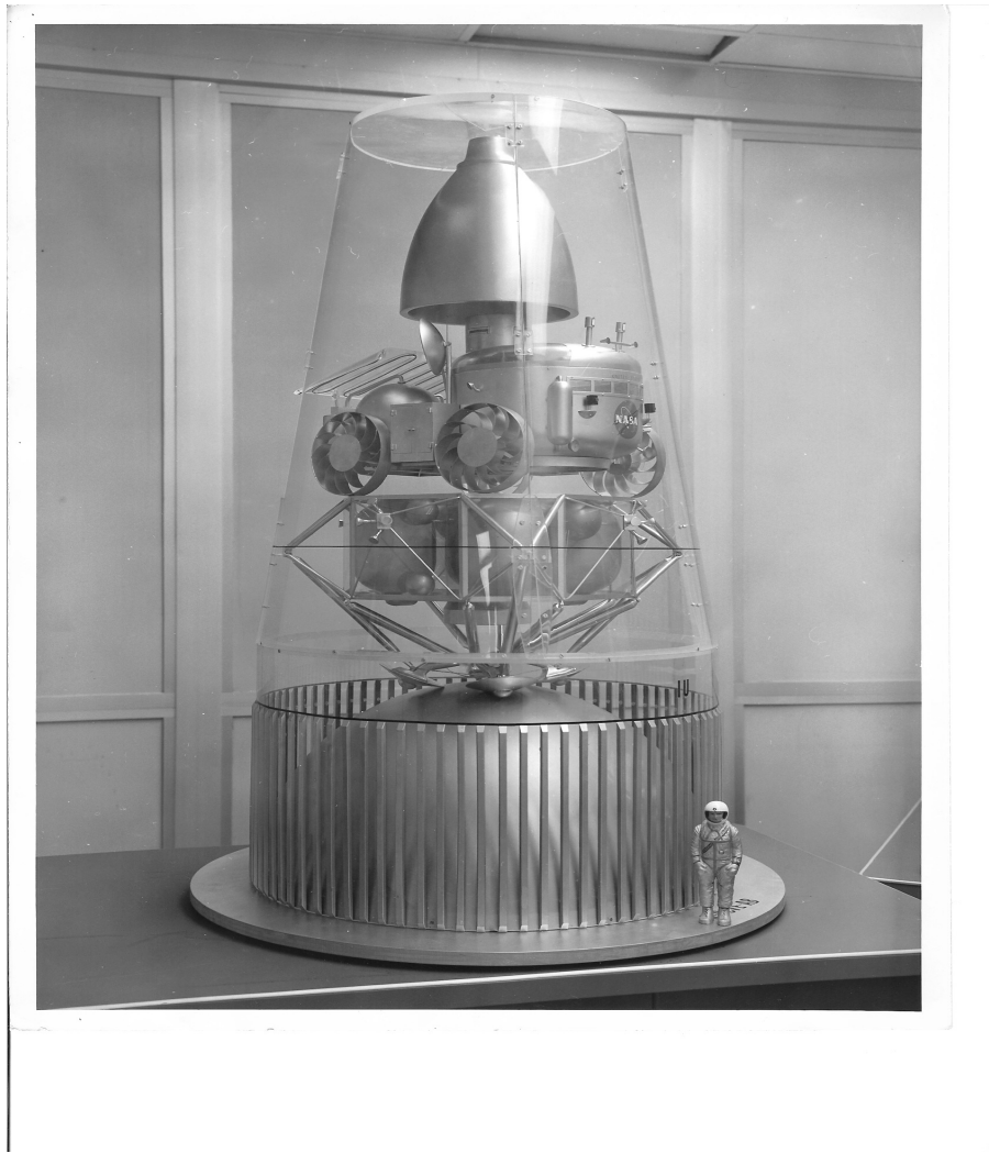
MOLAB Vehicle as stowed for transport to the Moon by the Saturn V.
