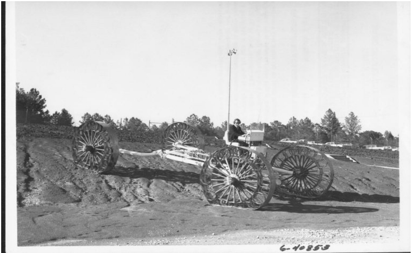
This is a photo of the Bendix Mobility Test Article that were developed for lunar mobility studies of large Lunar Rovers. It was also used for human factors and mobility evaluations here at MSFC.
