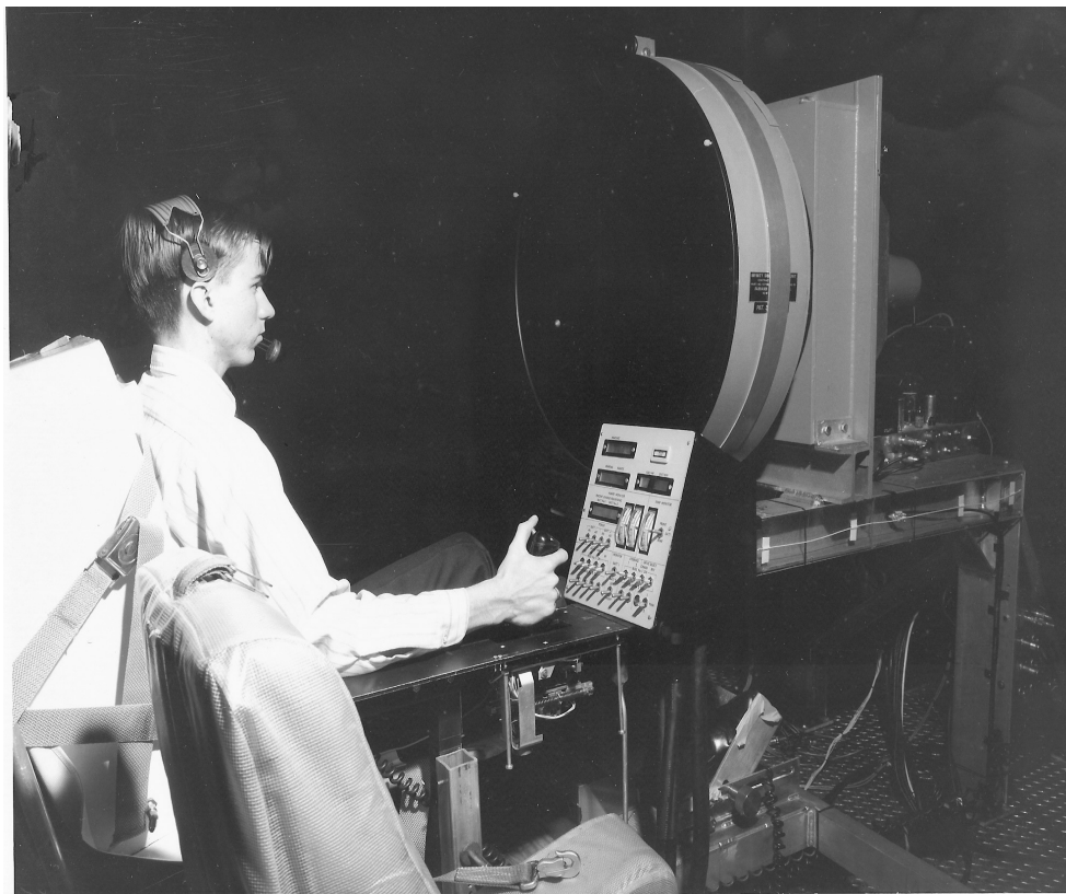
UnSuited Test Subject Driving the LRV Simulator with the large circular TV monitor display.
