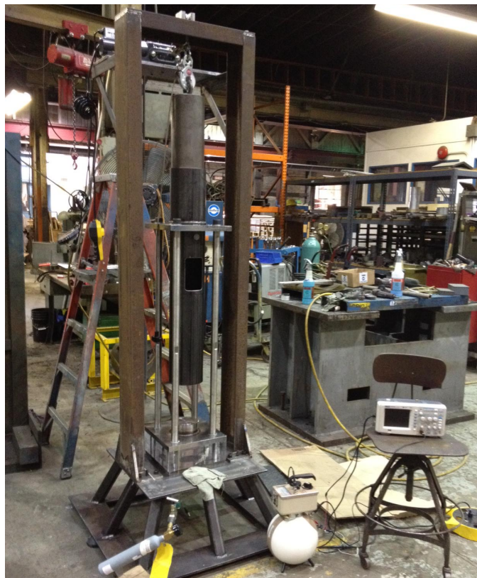
Fig. 15. The single-bubble cavitation-induced fusion experiment according to Smorodov (Smorodov, Galiakhmetov, & Il'gamov, 2008). After a deuterium bubble is injected into the glycerin the striker is released to impact the piston and create 300-500 bar pressure wave in the glycerin. The oscilloscope displays the signal from the neutron detector, which
