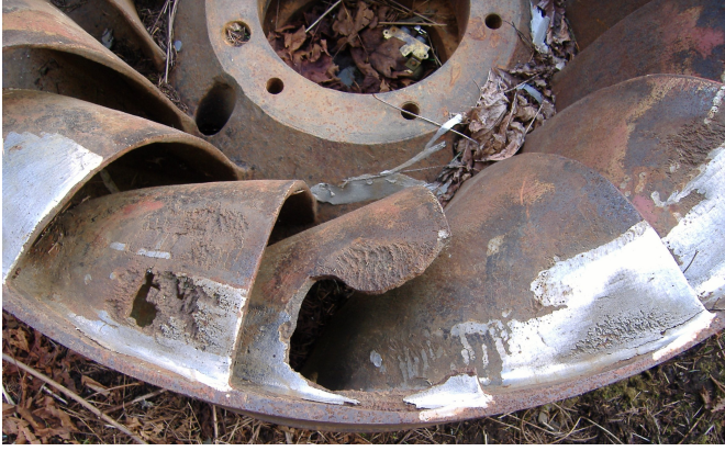
Fig. 2. Cavitation damage to a Francis turbine.
