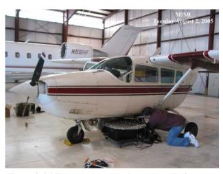
Figure 4 96-Element Antenna Array Installation
