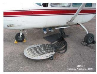
Figure 3 96-Element Antenna Array before Installation
