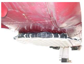
Figure 5 96-Element Antenna Array Mounted on the Aircraft
