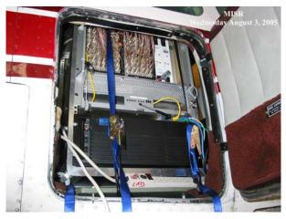
Figure 2 HAGR Receiver and Digital Recorder Installed on the Aircraft
