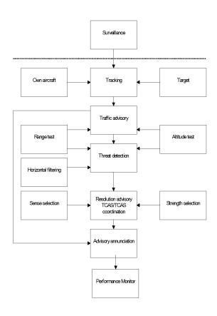
Figure 13. CAS Logic Functions
