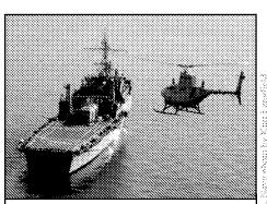
An RQ-8A Fire Scout (Group 4 UAS) Vertical Takeoff and Landing Tactical Unmanned Aerial Vehicle (VTUAV) System prepares to land aboard the amphibious transport dock ship USS Nashville (LPD 13).
