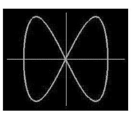
This shows the sine wave 90 degrees out-of-phase with the frequency of the horizontal sine wave three times the frequency of the vertical sine wave.
