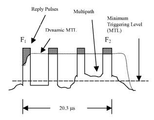
Figure 8. Dynamic Thresholding of ATCRBS Replies
