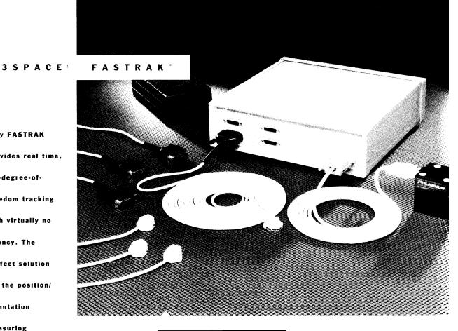
Only FASTRAK provides real time, six-degree-offreedom tracking with virtually no latency. The perfect solution for the position/ orientation measuring requirements of 3D applications and environments. Ideal for head tracking.
