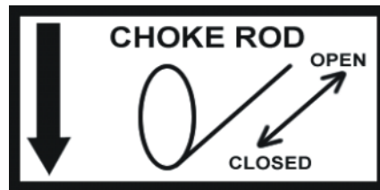
Figure 13- Pull choke out for closed position. Push in for open position.
