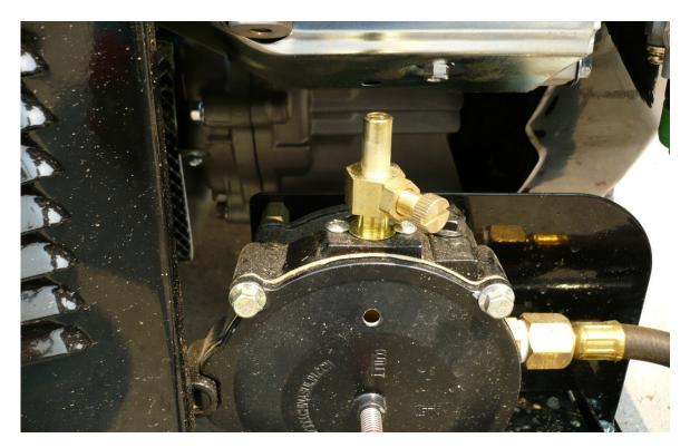
This is the fitting at the carburetor. It is the vertical brass tube with nothing connected to it now.
