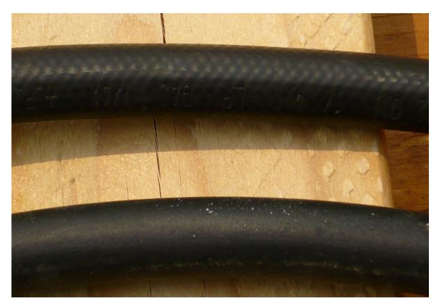
The long hose between the propane tank and the generator is marked. The 16" hose between the Pressure Regulator and the Carburetor has no markings.
