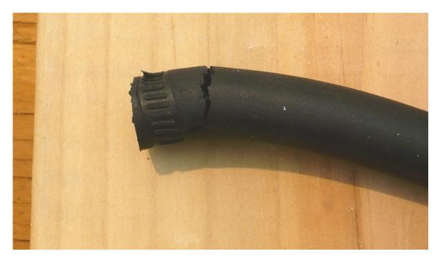
The hose on top is the long hose between the Propane Tank and the Generator. The hose on the bottom is the 16" hose between the Pressure Regulator and the Carburetor. Notice the difference.
